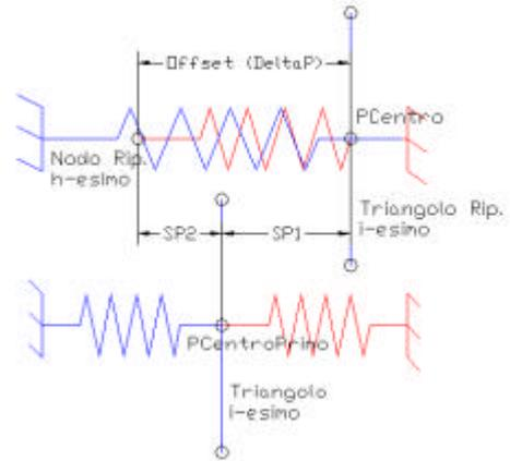
Figure 2. Equivalent model to simulate the node-triangle contact.
