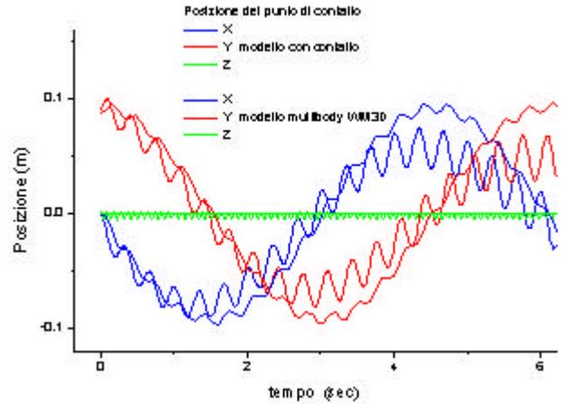
Figure 3. Comparison between spinning top simulation using numeric code and WM3D.
