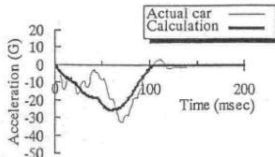
Figure 14. Acceleration during full frontal barrier collision (experimental and calculated in [2]).
