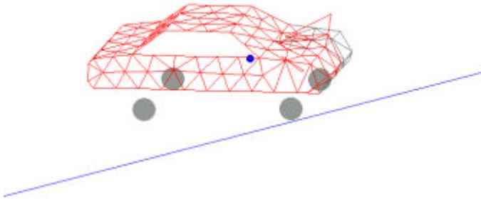
Figure 20. Deformed configuration of vehicle A.
