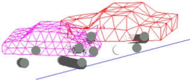
Figure 22. Overlap 50% offset collision simulation.
