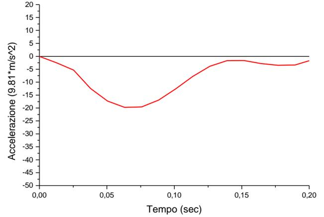
Figure 17. Acceleration in Overlap 50% offset collision (simulated).
