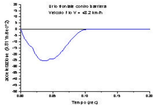
Figure 13. Acceleration during full frontal barrier collision (48.2 km/h).
