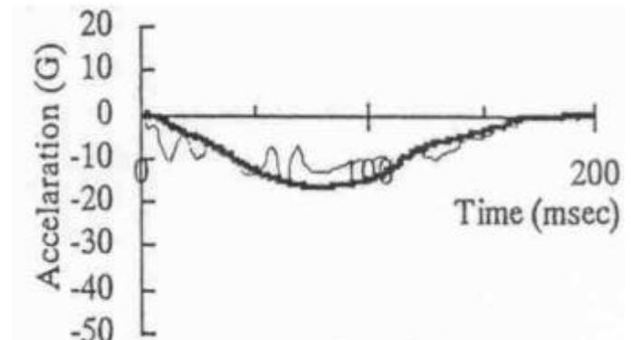
Figure 18. Acceleration in Overlap 50% offset collision (experimental and calculated in [2]).
