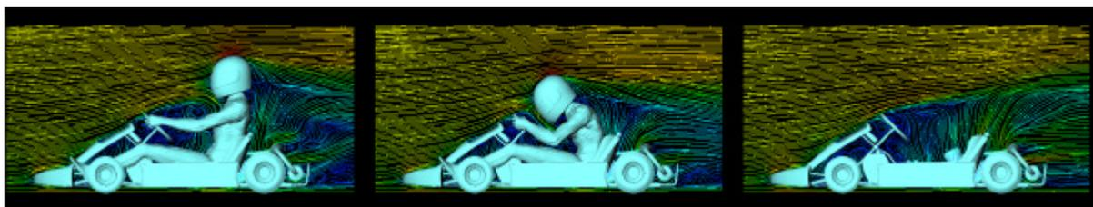
Figure 4. Aerodynamic simulations for two driver posture and no driver condition.
