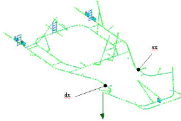
Figure 13: Static load testing: experimental layout; FEM model constraints and loads.
