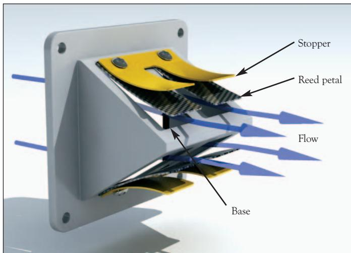
A diagram of a reed valve, showing the flexible reed petal, base, and stopper
