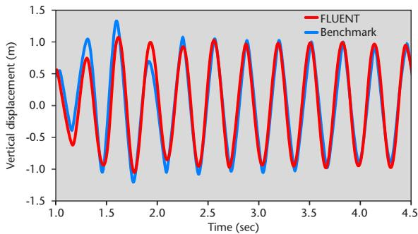
The vertical displacement of the beam free end predicted by the FSI model is compared to reference data (1, 2)
