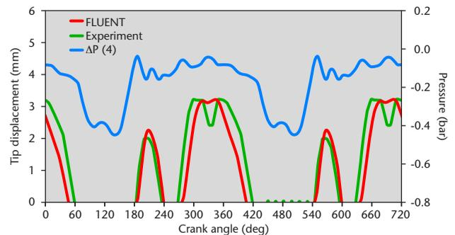
Tip displacement of an engine reed valve predicted by the FSI model and measured experimentally (4); the measured pressure differential is also shown
